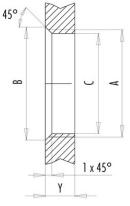
Installation direction: o-ring sits on chamfer.
